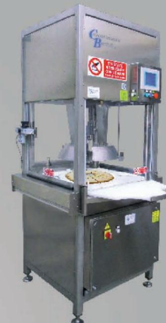
Automatic machine for fixed weight cuts. Rock 23
