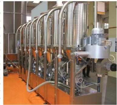
An electrical panel is on board of the station and together with a microprocessor control and manage the dosages of ingredients for each single recipe. In addition to this, it's also possible to use the Cepi managing software program to follow the whole process and have the traceability of raw materials by adding the bar-code system.
