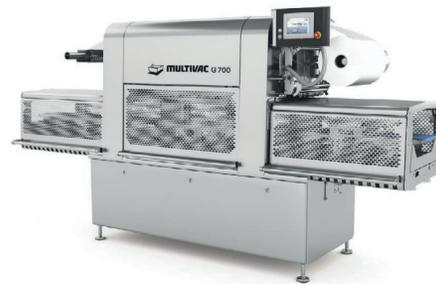
The Multivac traysealer G 700 is suitable for packing ready meals, snacks, vegetables and fresh-cut products of all types. Depending on the product to be packed, the G 700 can produce tray packs with or without modified atmosphere.
