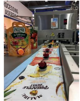
adapted to the different dimensions of the 'Pouch-up' bags by using its dedicated guides. The operating capacity is 400 bags/h for the AS-I-30 WEB filler and 800 bags/h for the AS-II-30 WEB filler. In both models, it is also possible to include a line to place the bags into the cartons automatically.
