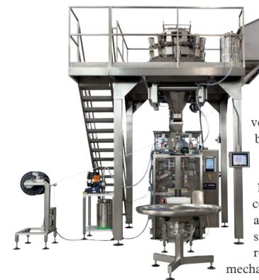
Vertical packaging machine with servomotors power supply system in DC bus voltage with energy saving, latest generation brushless servomotors with single-wire technology. Multilingual 10" Touch screen panel suitable for web connection with IP technology. Multihead weigher with framework in stainless steel AISI 304 and featuring new lowered-profile weighing modules with rear mechanics for easier cleaning.
