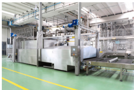
Automatic machine to wash, sanitize and dry horizontal trays
