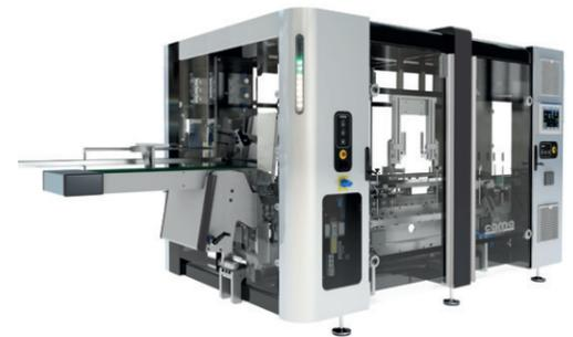
the carton boxes are moved towards the final closure station, which can work in continuous or intermittent mode.
