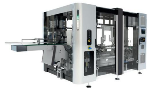
the carton boxes are moved towards the final closure station, which can work in continuous or intermittent mode.
