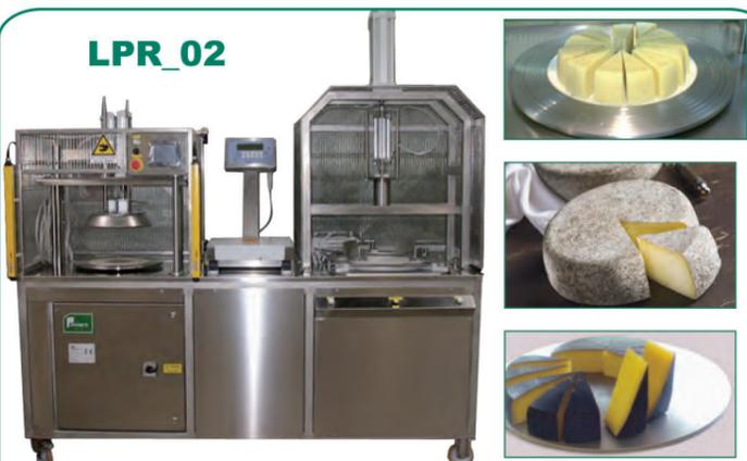
**Exact weight wedges semi-automatic cutter**
